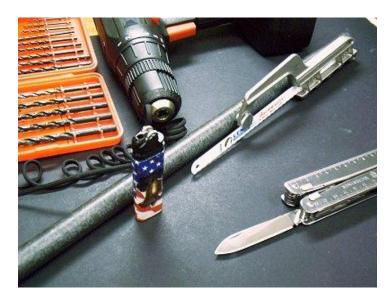
Please wear respiratory and eye protection when drilling and cutting material like this. You don't want to inhale things, such as Delrin and Nylon.
