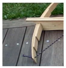
**Step 2**: Now you have to build the prod, which is the part at the front of the bow that stores the energy when the string is pulled back. Use a flexible 5 mm craft wood (it's up to you if you want to make them at home or purchase them) and cut strips of wood into three different sizes as it follows: 2 strips of 500 mm, 2 of 350 mm and another 2 of 200 mm.
