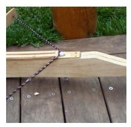
raises the washer higher than the arrow channel so the rope can slide off and launch the arrow.
