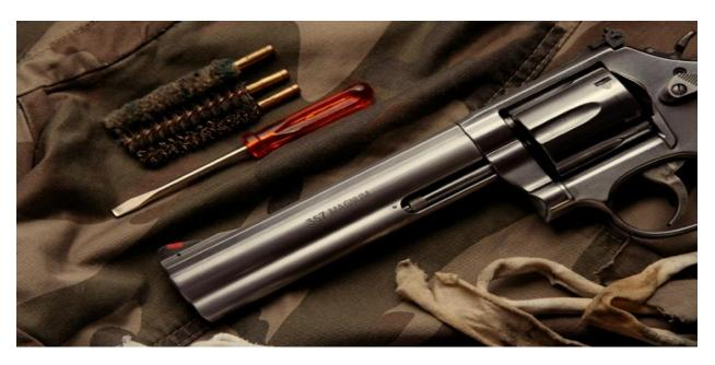
**Step 1**: Attach a bore brush to the cleaning rod and apply solvent on the brush. Push it back and forth through the bore several times. Add solvent to the brush as you work through. Once or twice should be enough.
